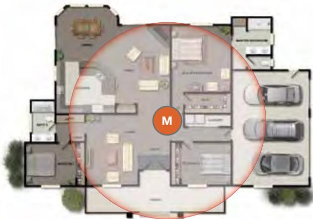
**Figure 9** Centrally locate the Master RF Base.
